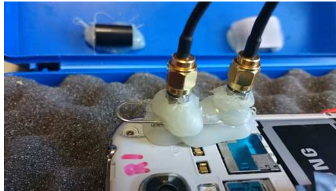
Figure 35 Samsung Galaxy S4 main and diversity internal antennas
