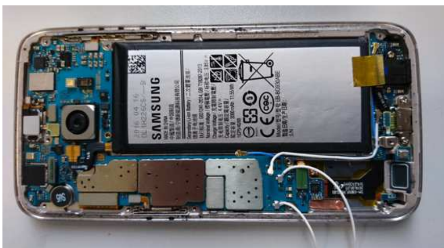
Figure 37 Samsung Galaxy S7 main internal antennas
