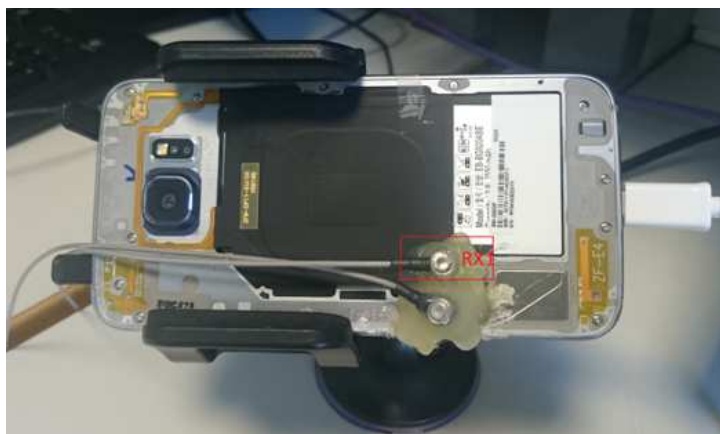
Figure 34 Samsung Galaxy S6 main and diversity internal antennas
