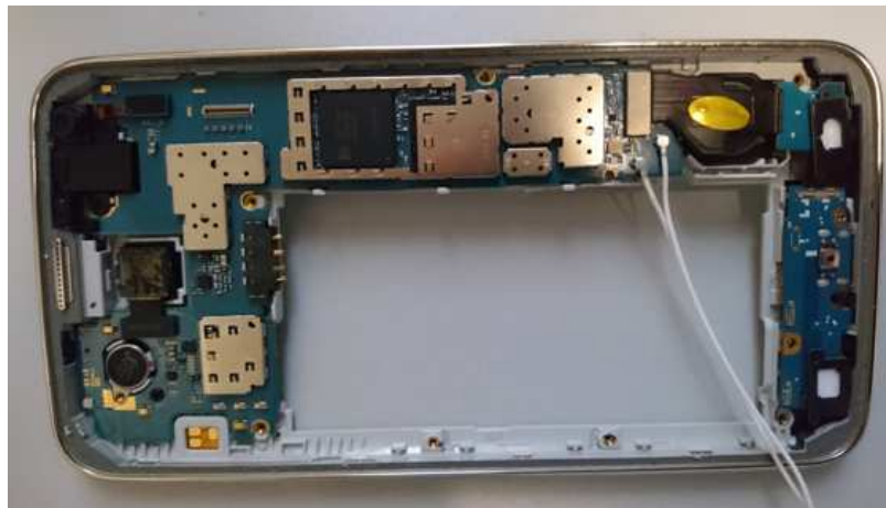
Figure 36 Samsung Galaxy S5 main and diversity internal antennas
