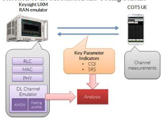
DL Channel emulator was used to model the channel influence by adding the noise (AWGN) and applying fading profiles defined in 3GPP specification such as (pedestrian, vehicular or high-speed train
